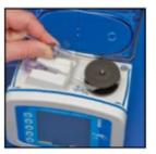
Grasp black ring retainer, gently wrap tubing around rotor, insert retainer directly into right pocket. DO NOT OVERSTRETCH TUBING.
